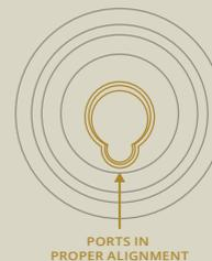
**\*\*\*It is important to make sure the ADAPT Module and main tube baffle ports are in alignment for maximum performance of your suppressor.\*\*\***
