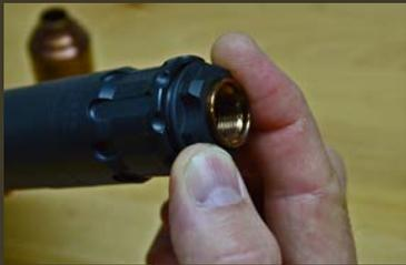
2. Remove the piston assembly from the main suppressor body.
