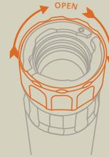
2. Hold the suppressor by the main body and thread suppressor onto the muzzle device until it is fully seated. Do not thread on using the locking collar.
