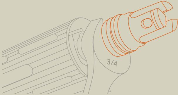
The use of a crush washer is prohibited due to improper bore alignment, which can result in baffle strikes.
