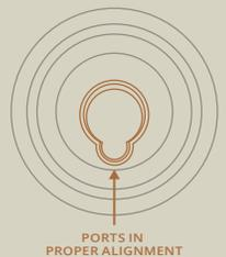
\*\*\*It is important to make sure the ADAPT Module and main tube baffle ports are in alignment for maximum performance of your suppressor. \*\*\*
