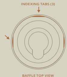
Each baffle has 3 indexing tabs for easy assembly.
